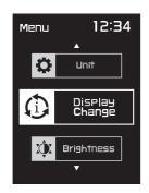
2. Push the "MENU" switch, use the select switch to highlight the display to change, and then push the "MENU" switch again.
