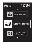
2. Push the "MENU" switch. The seat heater setting display will be shown and "High" will flash in the display.
