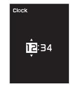
4. Push the "MENU" switch, and the minute digits start flashing.
