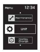
2. Push the "MENU" switch. The unit setting display will be shown and "L/100km" will flash in the display.
