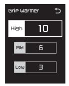
Push the "MENU" switch. The temperature level for the high setting will start flashing. Use the select switch to set the temperature level, and then push the "MENU" switch. "High" will start flashing.
