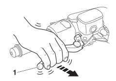
10.After the pulsating action has stopped in the front brake lever, it is generated in the rear brake lever "1" and continues for a few seconds.
