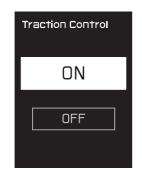
3. To set the traction control system to "OFF", push the select switch "✓" side for 2 seconds.
