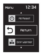
2. Push the "MENU" switch to exit the setting mode and return to the standard display mode.
