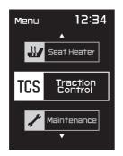
2. Push the "MENU" switch. The traction control system setting display will be shown and "ON" will flash in the display.
