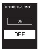
4. To set the traction control system to "ON" again, push the select switch " ^ " for at least one second.
